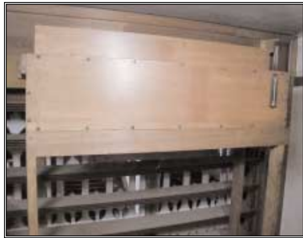
Original whiffletree motor in the Swell; swell shades behind
