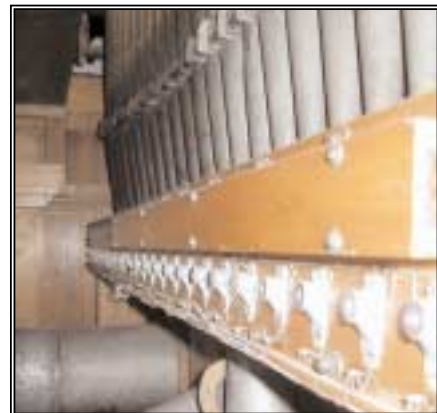
This offset windchest carries the tallest pipes of the Choir 16' Flûte conique. One valve muffler cover is in place; both magnet mufflers has been removed.
