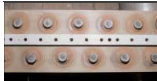
typical pouchrail inside a pitman windchest
