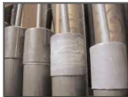
The original Swell Rohrflöte is now in use as the Pedal 4' Flute. "Rohr" is German for chimney, hence the thin tube atop each pipe. The canister caps have loosened with age. Shipping tape has been used to tighten this particular pipe.
