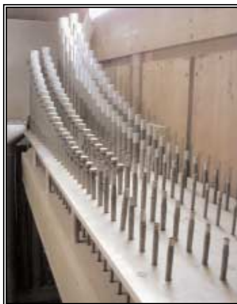
The added chest in the Swell, carrying the Nazard and Tierce pipes. This windchest was built by Reuter and installed in 1984.
