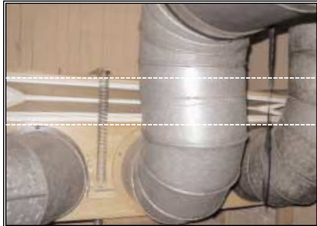
main static bellows (note unevenly rising top)
