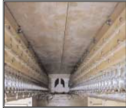
Key primary actions of the Pedal and upper Great pitman windchests. The mufflers have been removed. Note new magnets (shiny metal units)
