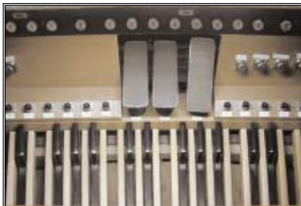
The pedal keys, toe terraces, toe studs and expression pedals appear original; newer toe studs have replaced the original kick pedals.
